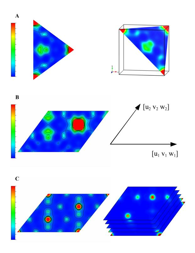
Figure 15.3: Electron-density distribution drawn with the three different modes for the (111) plane in rutile-type TiO<sub>2</sub>. (A) "(hkl) plane in the bounding box" mode, (B) "(hkl) plane defined by two vectors" mode, and (C) "Project along [hkl] axis" mode. The electron densities were determined by MEM from X-ray powder diffraction data.
