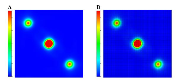
Figure 15.6: Electron-density distribution on the (001) plane in rutile-type TiO<sub>2</sub>. (A) without grid edges and (B) with grid edges drawn with solid lines.
