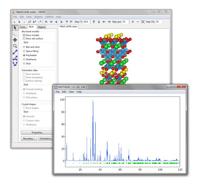
Figure 14.4: Simulation of an X-ray powder diffraction pattern of a high- $T_c$  superconductor, YBa<sub>2</sub>Cu<sub>4</sub>O<sub>8</sub> [88], which was plotted with Igor Pro.
